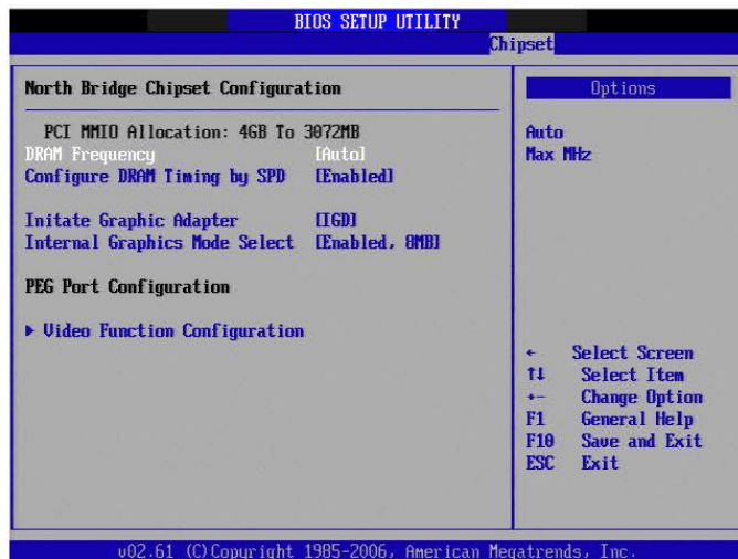
Figure 3.24 North Bridge Configuration
